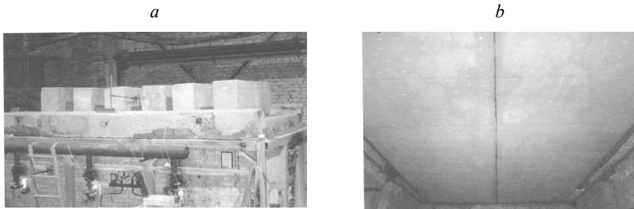
Fig. 1. The view of floors before testing (a) and samples from the furnace side before testing (b).
