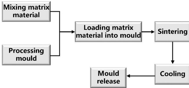
Figure 1. Fabrication process of drill bits
