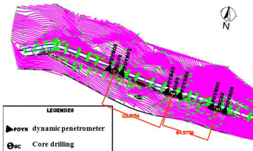
**Fig.4.**Plan view of the site with implantation of the drilling investigation (Zemouri& Arab, 2012) amended.
