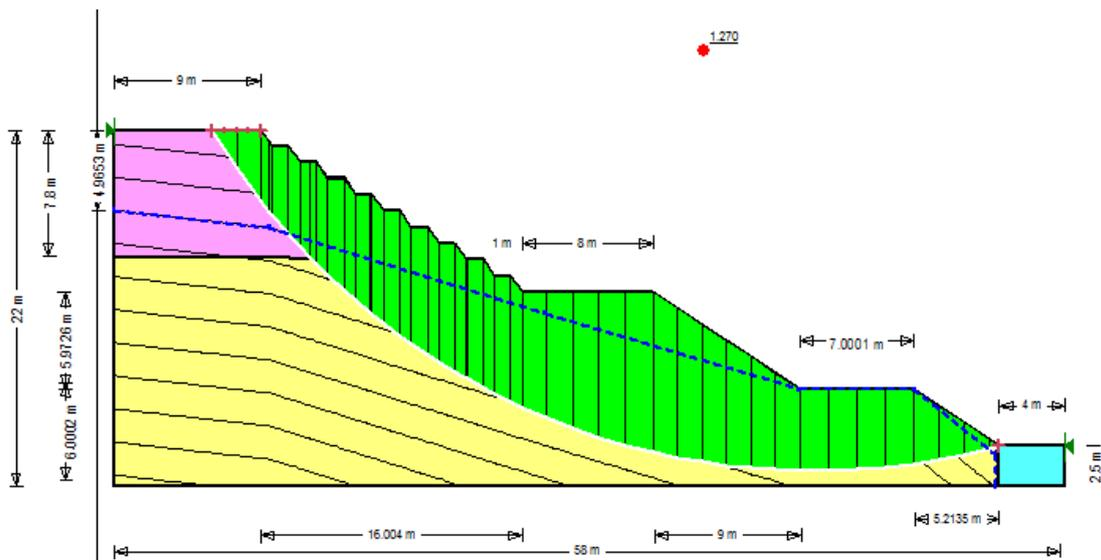
Fig. 5. The critical slip circle around the slopes after reprofiling in the dry period (result calculated by the method of Fellenius)
