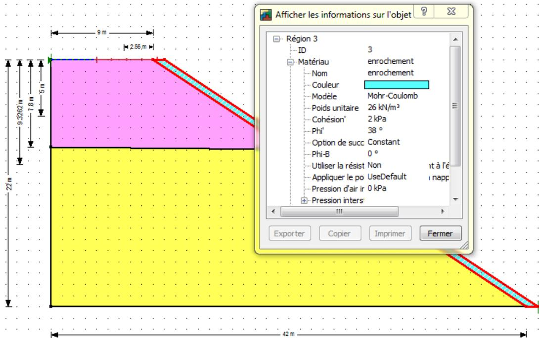
Fig.4. Property of the rock material used for the mask
