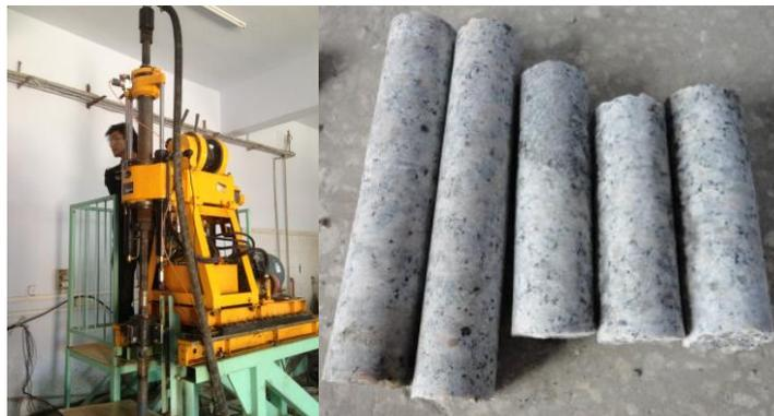
Figure 3. XY-1 core drill rig Figure 4. The core taken out by drilling experiment
