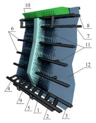
Fig. 1. 3D version of technological scheme of fans of wells arrangement during stoping operations conducting with application of explosives emulsion for ore deposits with thickness of 5–25 m:
