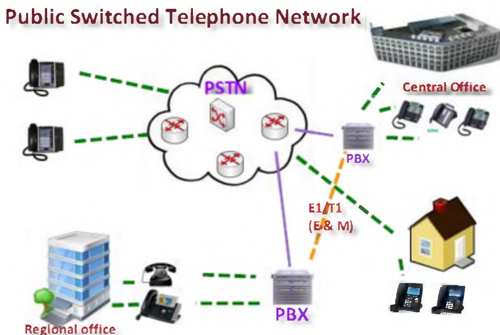
Рисунок 1.1 - Public Switched Telephone Network
