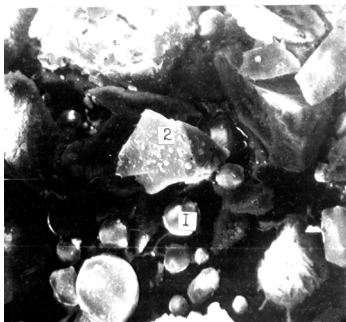
Fig. 1. General view of TPP ash particles (initial), magnification 517x: 1 – spheres; 2 – coal particles.
