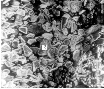
Fig. 3. General view of TPP ash particles (after treatment with 40% H_2SO_4 ), magnification 1305x; 2 – coal particles.
