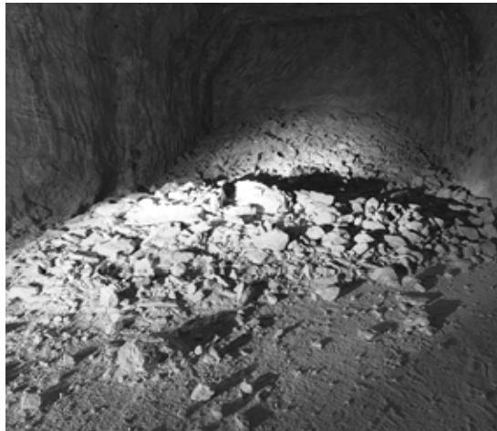
Figure 10 – Blast results with Rioper G permissible explosive type
