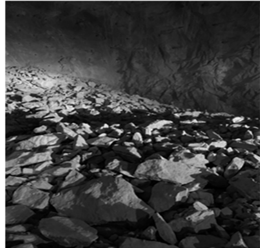
Figure 8 – Blast results with Emulinit PM permissible explosive type
