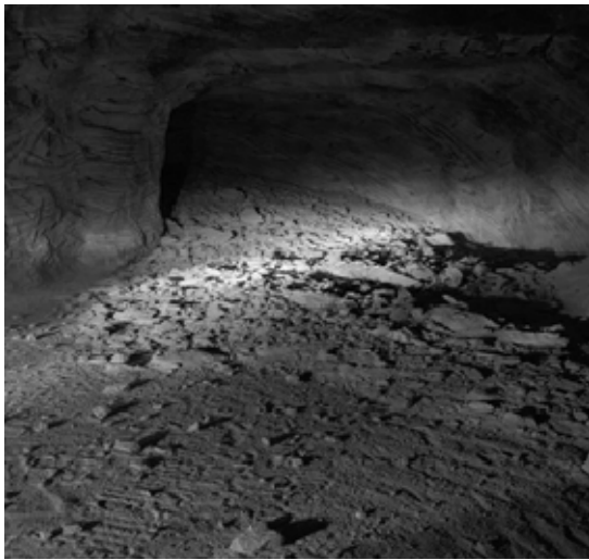
Figure 4 - Blast results with Ammonex 3 explosive type
