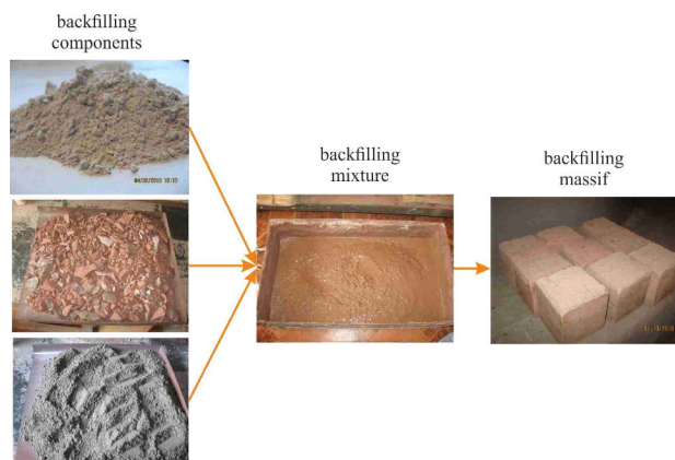
Fig. 2. The sequence of the backfill massif formation under laboratory conditions
