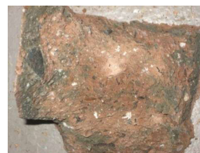
Fig. 3. The examined surface of a fracture specimen of the backfill massif
