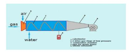
Using the installation it is possible to determine the influence of the magnetic field to parameters change during natural gas combustion.
