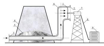
**Fig. 5.** Operation schedule to utilize energy of technogenic air flow while using heat generated by mine dumps: 1 - windwheel of a wind-driven power plant; 2 - diffuser; 3 - heat-generating pipe; 4 - mine dump; 5 - zone of active oxidation of the mine dump organic mixtures; 6 - thermal protection of the diffuser; 7 - electric generator of the wind-driven power plant; 8 - electric cable; and 10 - control box.
