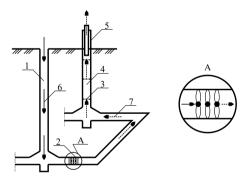
**Fig. 1.** Procedures to use energy of technogenic air flows within underground mine workings by means of wind-driven powerplants: 1 - supplying ventilation shaft; 2 - block of wind-driven powerplants of a development mine working; 3 - wind-driven powerplants of a shaft; 4 - ventilation shaft; 5 - overshaft tubular helium air heater; 6 - fresh air; and 7 - dusty air.
