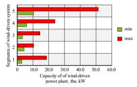
**Fig. 8.** Monthly electrical energy generation by certain segments of wind-driven system: 1 - wind-driven generators of technogenic air flows of mine workings; 2 - wind-driven generators of air flows of a mine shaft; 3 - wind-driven generators mounted on a main mine fan; 4 - wind-driven generators of thermal technogenic air flows of a mine dump; 5 - wind-driven devices of mine dumps, thousand.
