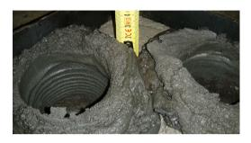
**Fig. 4.** The view of the melt (plaster stone) obtained at a rotation frequency of 500 min<sup>-1</sup> and an axial load equal to 700 daN, for TPCM with a component ratio of 1:3.
