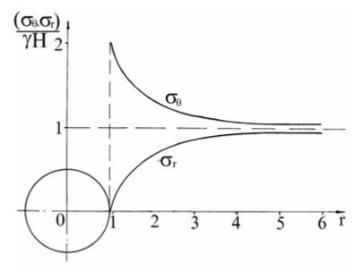
Fig. 4.2. Stress distribution around excavation in the rock mass
