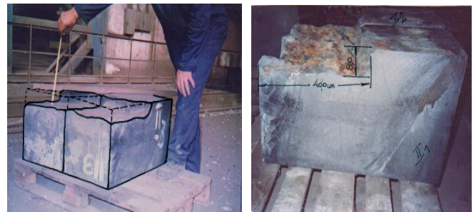
Figure 6. Measurement of dissolution of graphite blocks II3 and II1 in contact with a metal with a low C-content
