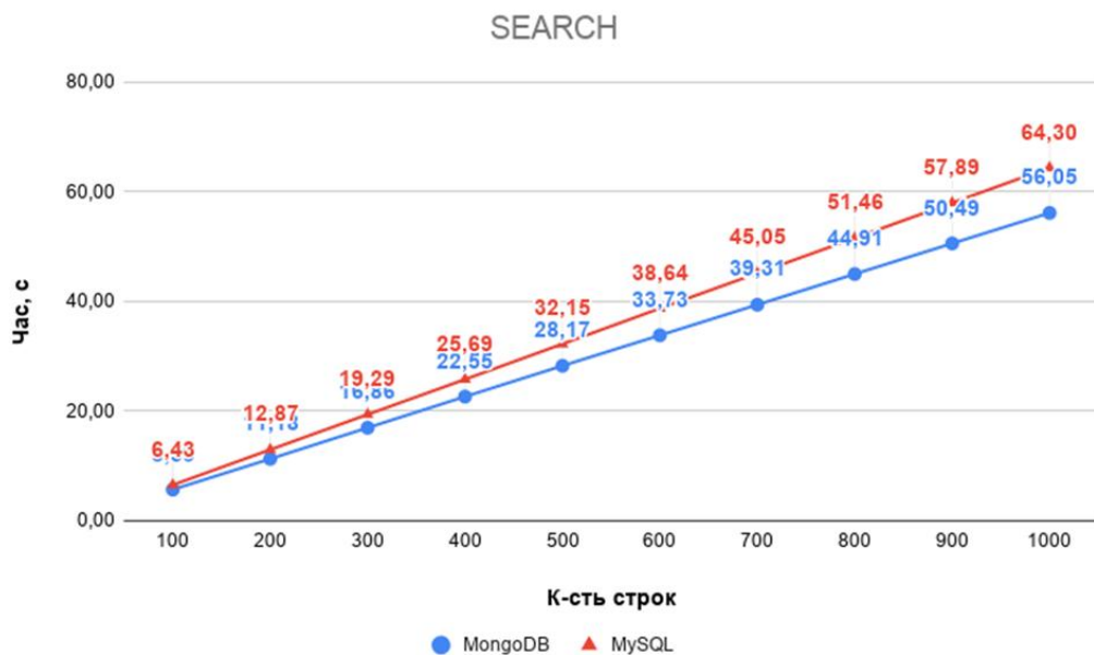
Fig. 2. Diagram of the execution time of a SELECT operation (not index) on the number of entries
