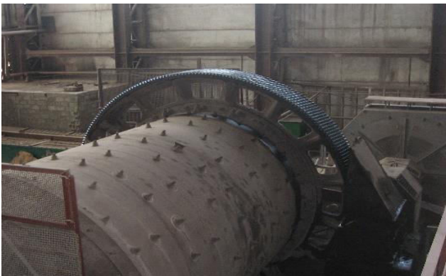
Figure-2. The Ball Mill of the MShTs 36×55 type for wet grinding of the granulated blast-furnace slag.
