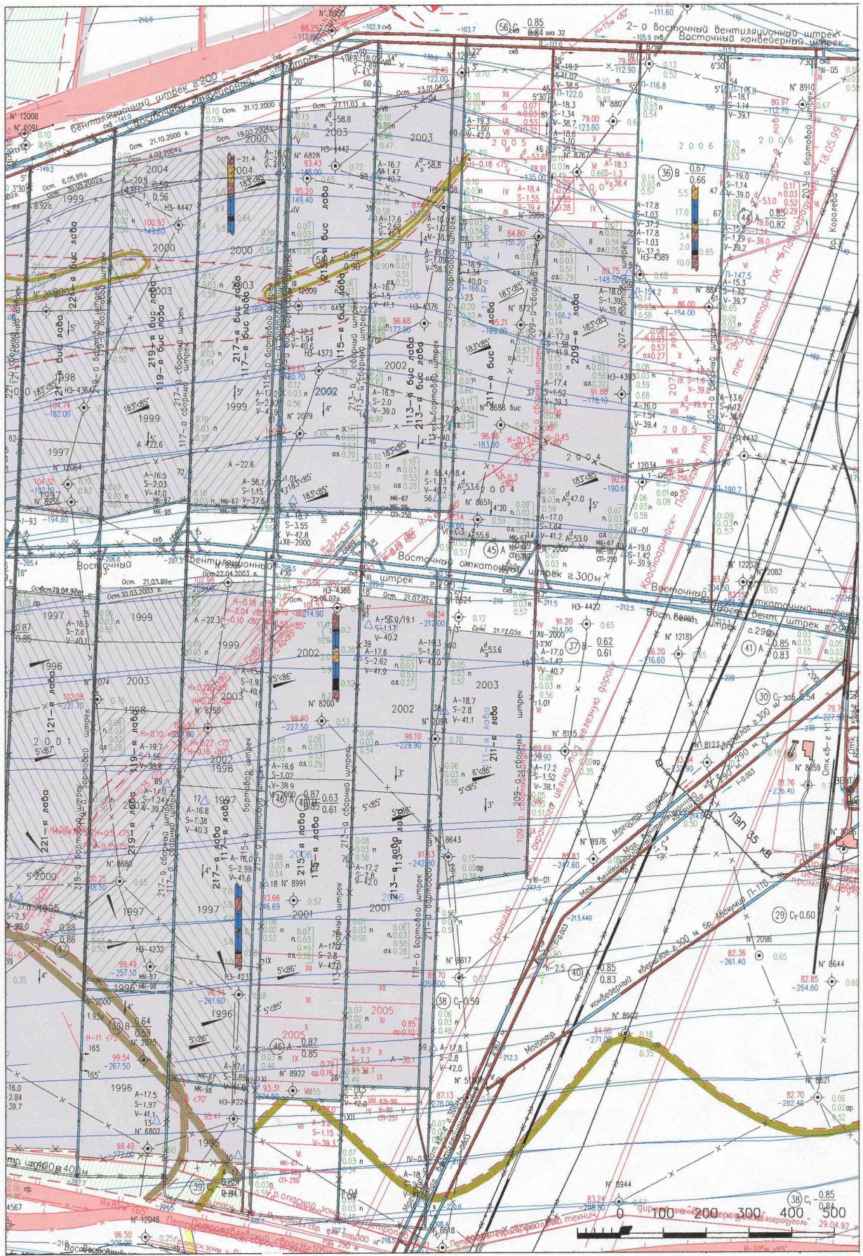
Fig. 4.4 Integrated mining plan in the context of C_6 and C_6^1 seams
