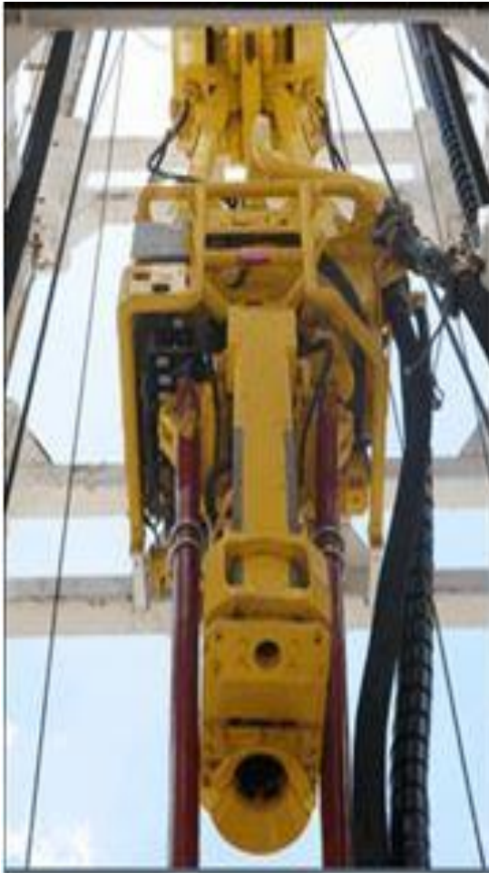
Figure 2.6 - The Top Drive System
