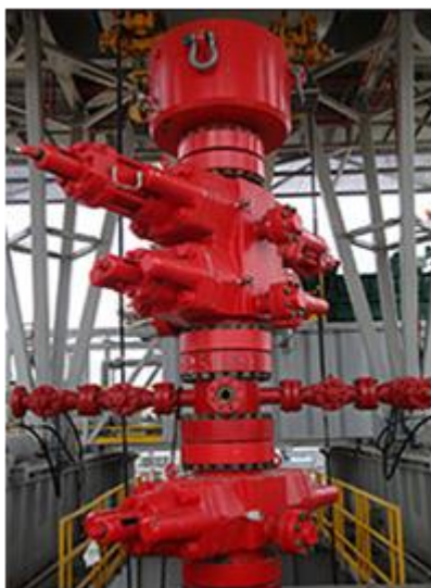
Figure 2.13 - Land BOP A Subsea BOP Stack
