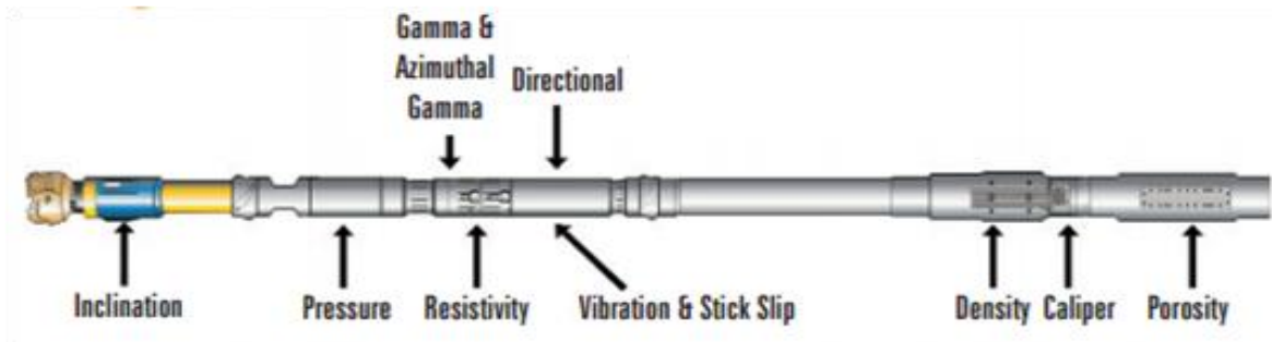
Figure 2.17 - A Typical Geosteering BHA (from Baker Hughes)
