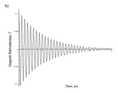
It is energetically more advantageous to demagnetize magnetite in a pulsed mode. For this, damped oscillations of the required frequency are excited in an oscillatory circuit formed of a solenoid and a capacitor. In this case, all particles inside the solenoid are demagnetized. What is more, the pulse repetition interval should be less than the period, when the suspension is in the solenoid (see Figure 2, a).
