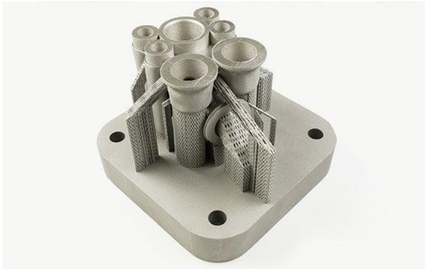
Figure 2.5.4 Example of a part on the build plate with support structures
