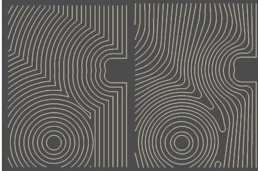
Figure 2.7.1 Example toolpaths for conventional milling (left) and HSM (right)
