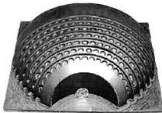
Figure 2.4.1 Graphite electrode after HSM, size 350 \times 200 mm; 9600 hexagonal holes with a radius of 0.2 mm; outer surface treatment with a 10 mm ball mill; hole treatment with a 1.5 mm roughing mill; finishing with a 0.4 mm mill; spindle speed 45,000 min -1 , processing time 34 hours.
