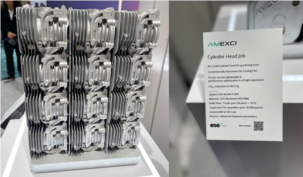
Figure 1.4.2, Cylinder Heads printed on EOS M300-4 1KW
