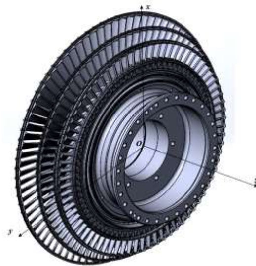
Figure 1 – The 3D model of the gas turbine rotor as a solid body
