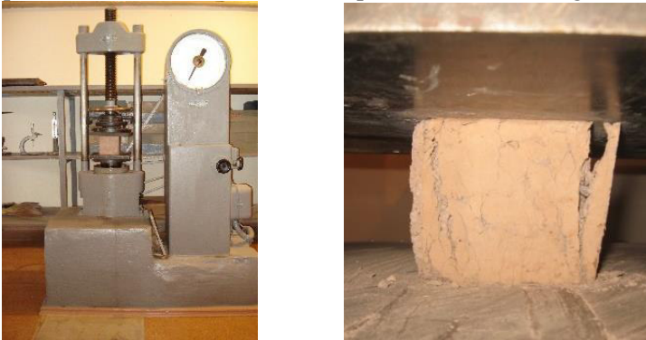
Fig. 5. Strength test of hardening backfill mass samples
