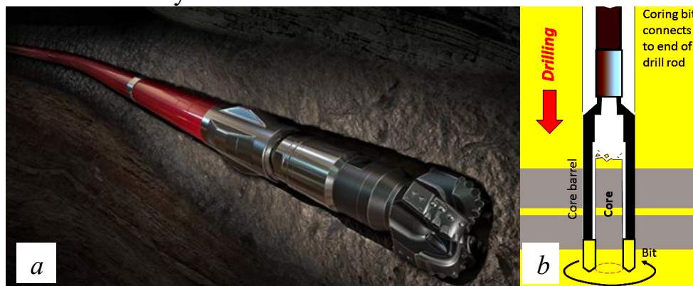
Figure 1.1 Schemes of drilling wells by continuous ( a ) and annular ( b ) face
