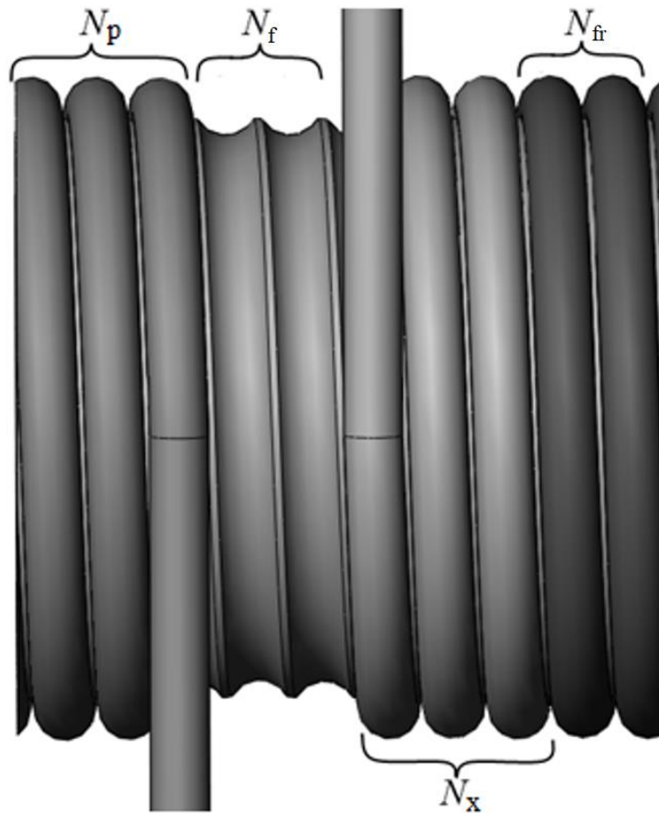
Fig. 2.1. Model of the distribution of turns on the wedged part of the MHM drum
