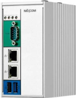
d) IoT gateway by Nexcom (CPS-100-M model)
