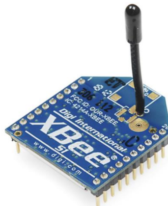
Fig. 4.17. The external view of a typical ZigBee module
