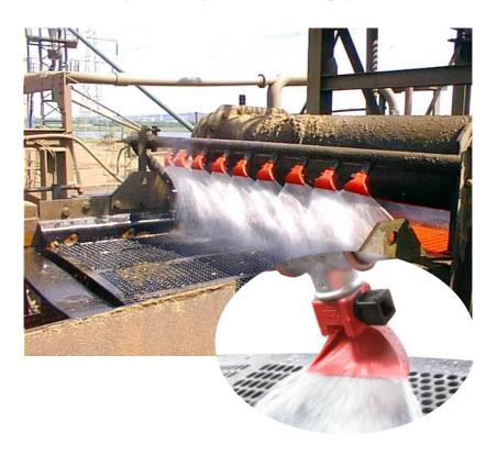
**Conclusion.** The entire cleaning procedure takes a few seconds, and does not require the workflow stop. Sprayers are made of high-strength plastic that completely excludes corrosion. Simple threaded fastening with external thread 3/4".
