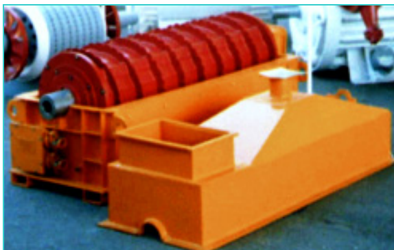
Figure 2. A general view of the auger PEEC with removed upper part of casing
