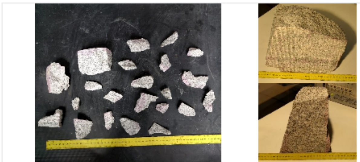
Figure 3.4-2 Pieces, created as a result of failure of the sample
