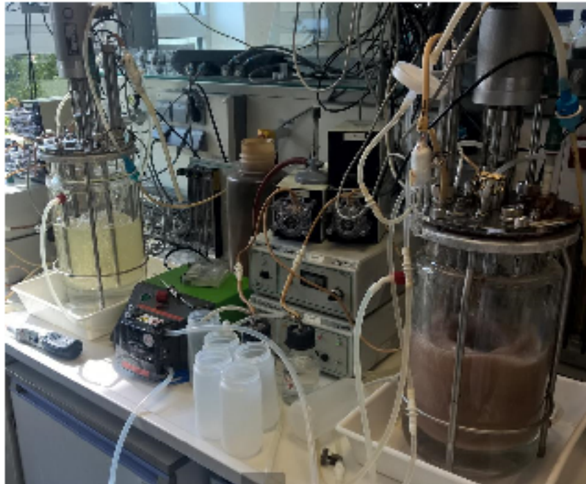
Figure 9 \gamma -PGA production by B. licheniformis DSM 8785
