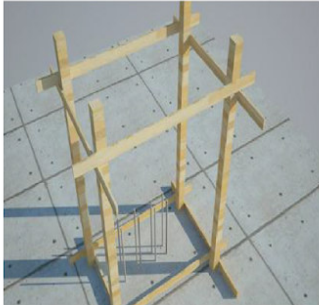
Figure 3.13. Formwork of columns.
