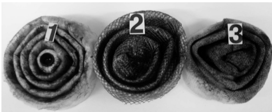
Fig. 2.51. Filters of “Astra-2” respirator made of eleflen (1); made of \Phi\Pi\Pi 15-0,6 on meshwork (2); made of \Phi\Pi\Pi 15-0,6 with gauze backing (3)
