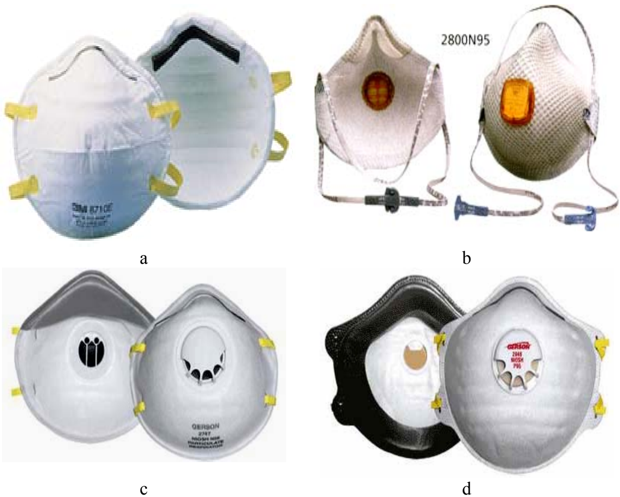
Fig. 2.11. Obturation line designs: a is respirator by 3M without gasket along obturation line; b, c are rubber gasket and polyurethane strip round nose bridge (respirator by Willson); d is polyurethane strip all along obturation line (respirators by Willson)
